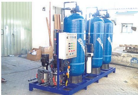
30 GPM Filtration, Dubai
